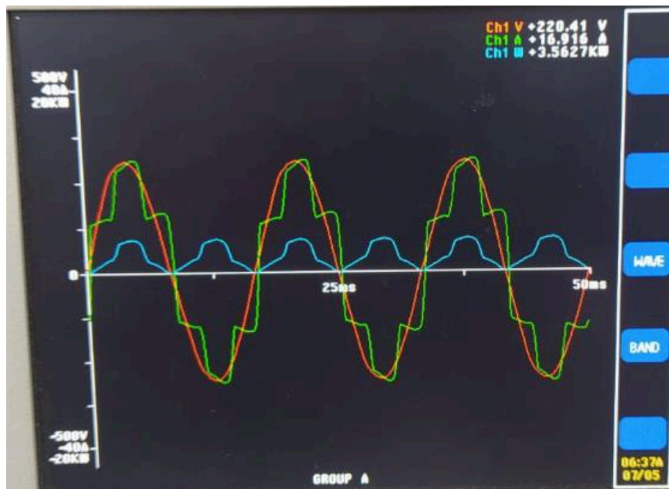
Figure 16 – Demonstration of the waveform without the filter.
