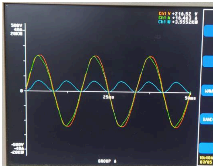
Figure 19 – Demonstration of waveform with the filter.
